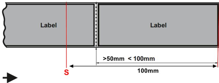
**Picture 7.3:** in scenario C the correct stop position is 100mm minus the label length minus 1/2 gap length
