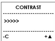
By pressing the M-key, the desired value is saved and the display switches to the brightness settings. You can now also adjust the brightness with the "C" and Δ buttons.
