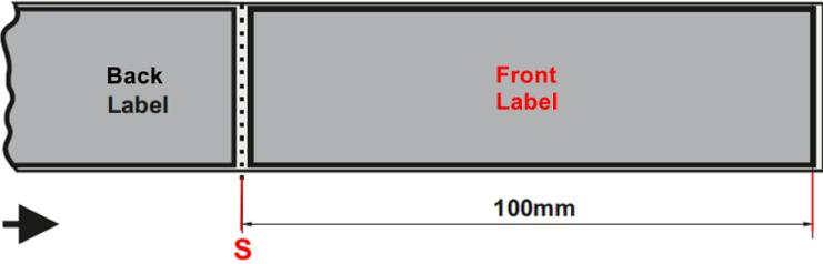
**Picture 9.2:** in scenario B the correct stop position of the front label is 100mm.
