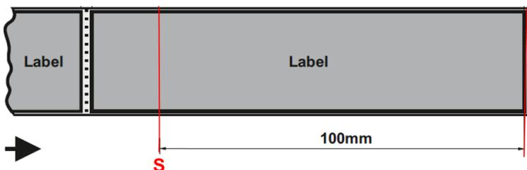
**Picture 7.1:** in scenario A the correct stop position is 100mm.
