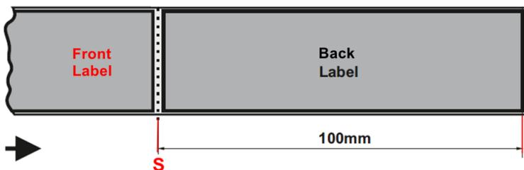
**Picture 8.2:** in n scenario B the correct stop position of the back label is 100mm.
