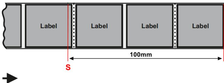
**Picture 7.4:** in scenario D the correct stop position is 100mm minus the combined length of all the labels and all the gaps, plus 1/2 gap length.
