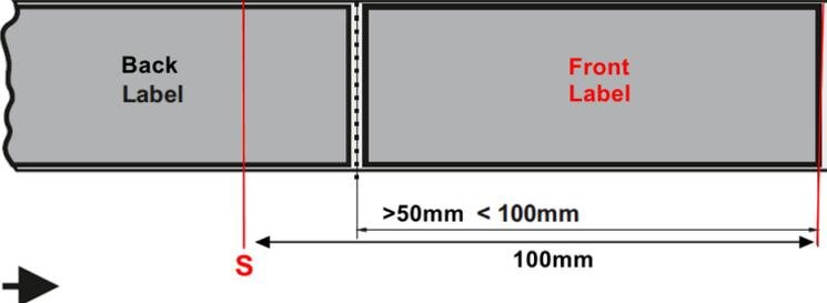
**Picture 9.3:** in scenario C the correct stop position of the front label is 100mm minus the label length minus 1/2 gap length
